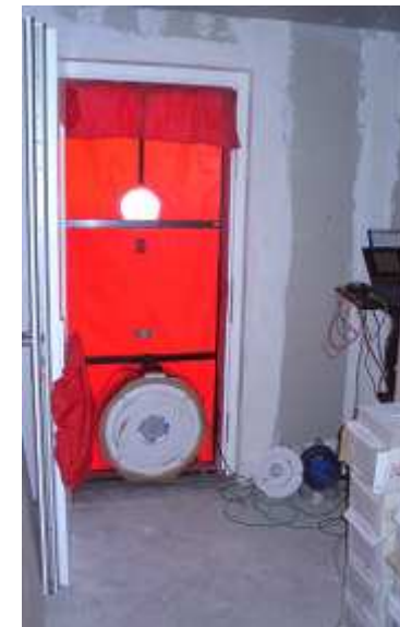
Fig. 3. 23 – Blower door installed for a pressurization test
