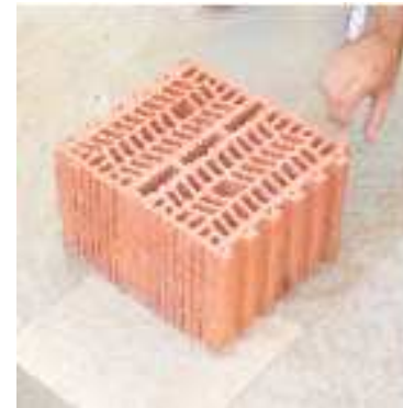
Fig. 3. 19 – Porous ceramics brick as used in a passively cooled project in Seville
